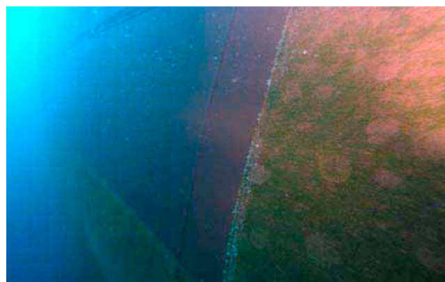
Figure 3. Ship's hull after 25 months of navigation at 13 knots average speed with 60% activity. The patch covered with silicone hydrogel is clean, whereas the hull coated with SPC copper-based paint is fouled by algae and slime. [Reproduced from ref 37, with kind permission.]
